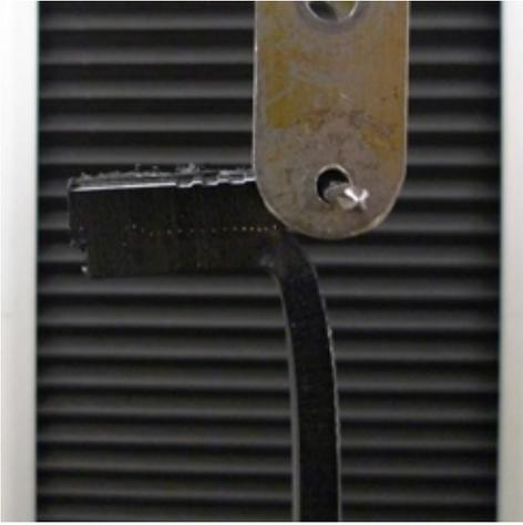
**Figure 1.** Peel test setup as per ISO 13954
